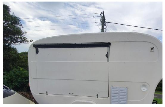
Note that when filling the tank it will **overflow** when full under the caravan. Once this starts happening **stop filling immediately**. Also smart to use the pump tap inside about 5- 10 pumps if you have overfilled it to ensure less chance of leaking once travelling.
